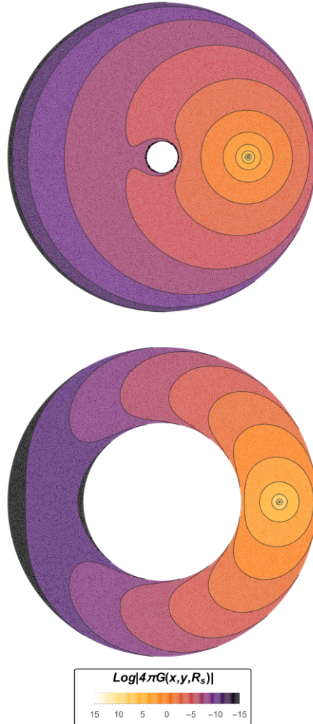
Figure 4.3: Density plot of the Wightman function given by Eq. 4.1 with \zeta = 0 for two representative values of radii (a) a = 10 and b = 20 ; (b) a = 10 and b = 100 . The represented plane crosses the source charge and the center of the spheres. The Wightman function is null at the surfaces, satisfying the Dirichlet boundary conditions and diverges over the source charge.
