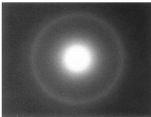
Figure 2.11: Electron-diffraction pattern, a diffusive ring, of the smectic-A phase.
